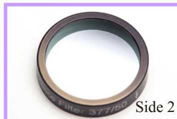
Semrock DAPI Exciter After > 1000 hrs
