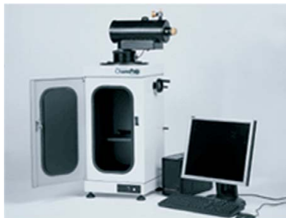
Chemi-Luminescence Image System
