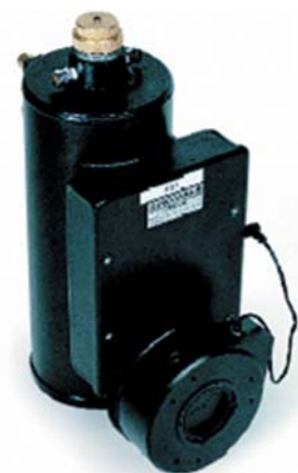
LN Cooled CCD Camera
